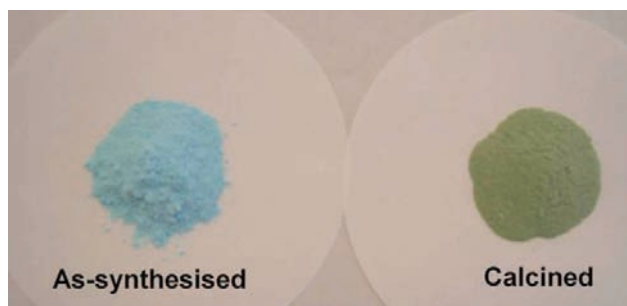
Fig. 3 As-synthesised and calcined CuAPO-5, colour change indicative of change in copper environment
