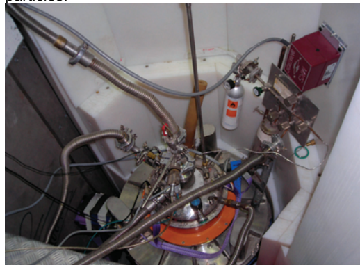
Sample and cryostat placed in the neutron beam. Photo: Astrid Lund Ramstad.
