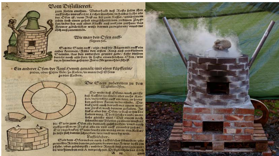
Figure 1: To the left one page from Lonicer's Kreuterbuch . To the right a reconstructed and working distillation furnace in Norway in November, as described in Lonicer's Kreuterbuch . Some of its paraphernalia are visible through the vapour such as specially shaped bricks, "Moor's head" of reticulum, gasket of intestines, curcubit and helmet, as well as the "starke wasser" nicely distilling from the beak.
