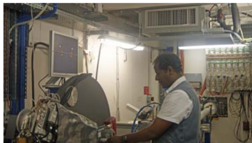
Fig 3. High resolution XRD experiments being conducted on some of the painting samples at section BM01B of the SNBL.
