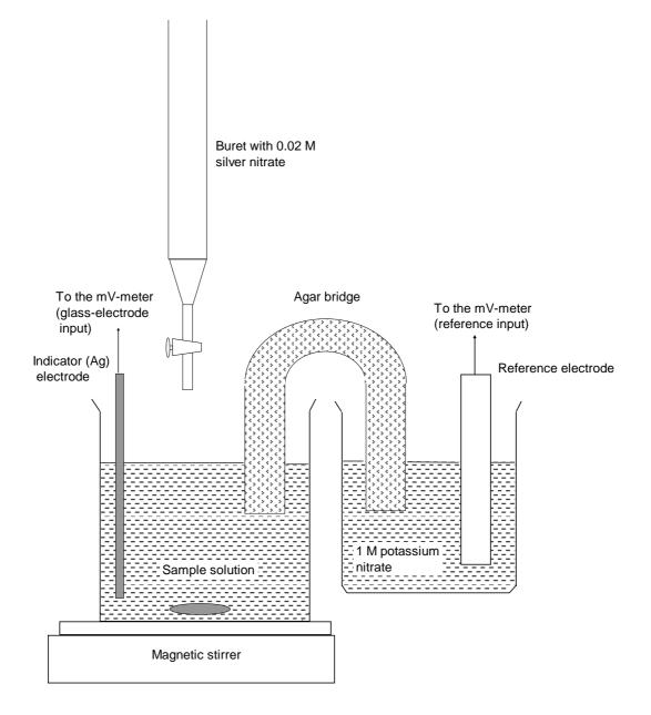
**Fig. 1.** Schematics of the experimental set-up for potentiometric titration by a silver nitrate solution.
