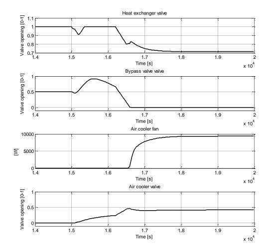
Figure 6.20: Manipulated variables. Switching from  $\alpha$  to  $\beta$ .
