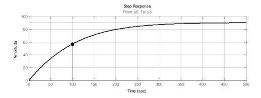
Figure C.1: Open loop step response for air heater.
