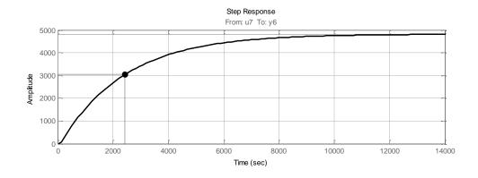
Figure C.2: Open loop step response for Air cooler – frost protection.
