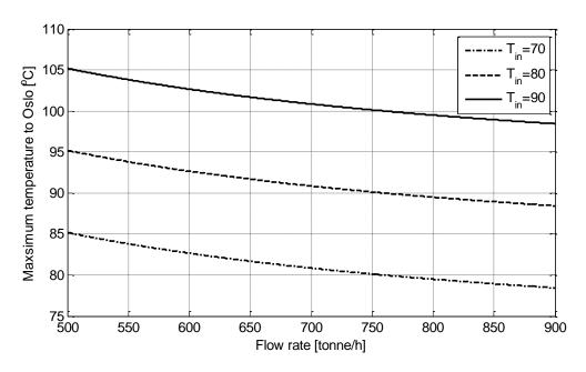
Figure 6.2: Maximum outlet temperature,  $T_{out}$  as a function of flow rate.
