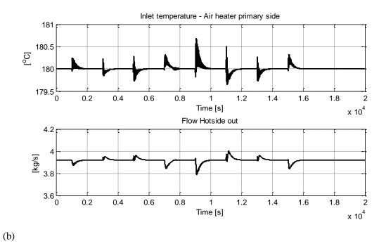
Figure 6.6: Air temperature towards the furnace and disturbances.
