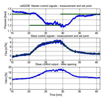
Fig. 14. Cascade PI control of top pressure and volumetric flow: step responses in closed loop.
