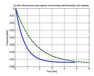
Fig. 4. Asymmetric flow line pressure response with 1% increased (solid) and 1% reduced (dashed) choke. Note that the response for the reduced valve opening is inverted in the figure.
