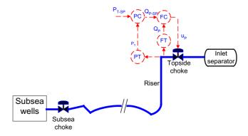
Fig. 5. Top pressure and volumetric flow cascade control.
