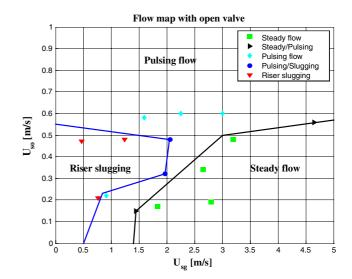
Fig. 8. Flow map with 100% open choke. The superficial gas velocity  $U_{sg}$  is plotted along the *x*-axis and the superficial oil velocity  $U_{so}$  is plotted along the *y*-axis.
