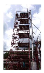
Fig. 6. The 15m high riser at Tiller with the control choke at the top.
