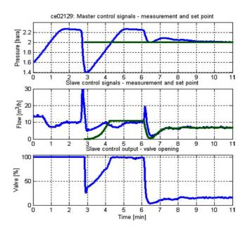
Fig. 10. Cascade PI control of flow line pressure and volumetric flow: slug suppression.
