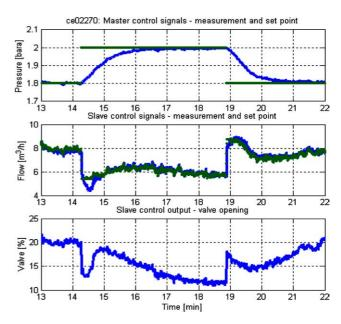
Fig. 11. Cascade PI control of flow line pressure and volumetric flow: step responses in closed loop.
