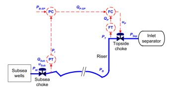
Fig. 3. Cascade control of flow line pressure  $(P_i)$  and volumetric flow  $(Q_P)$ .
