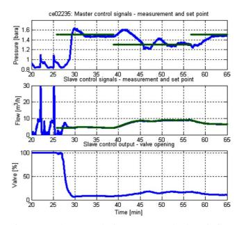
Fig. 13. Cascade PI control of top pressure and volumetric flow: pressure at the top with set point, volumetric flow with set point and choke opening.
