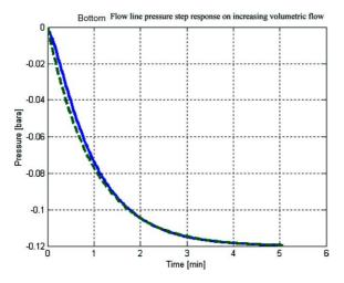
Fig. 9. Flow line pressure step response (solid) and linear approximation (dashed).
