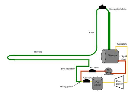
Fig. 7. Schematic overview of Tiller medium scale multiphase experimental loop.
