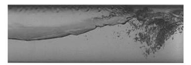
Fig. 1. Lab photo of multiphase slug flow. The picture is by courtesy of Sintef Petroleum Research.
