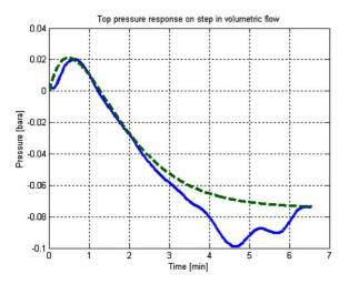
Fig. 12. Top pressure step response (solid) and linear approximation (dashed).
