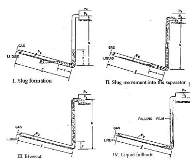
Fig. 2. Schematic view of riser slugging cycle.
