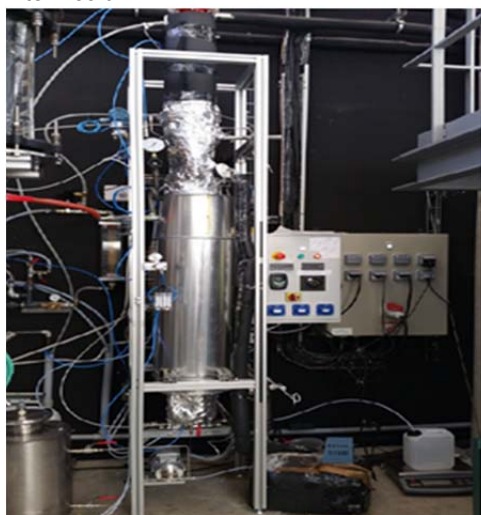
Figure 3: Experimental set-up of heat transfer validation.
