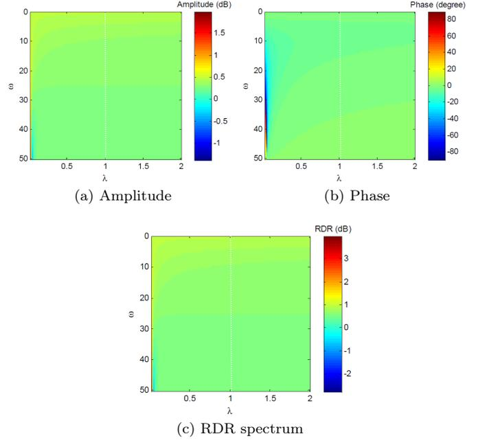
Fig. 3. Frequency characteristics of the controllers for  $\omega \in [0, 50]$  with an increment of 0.1rad/s versus  $\lambda \in [0, 2]$  with 0.002 increments
