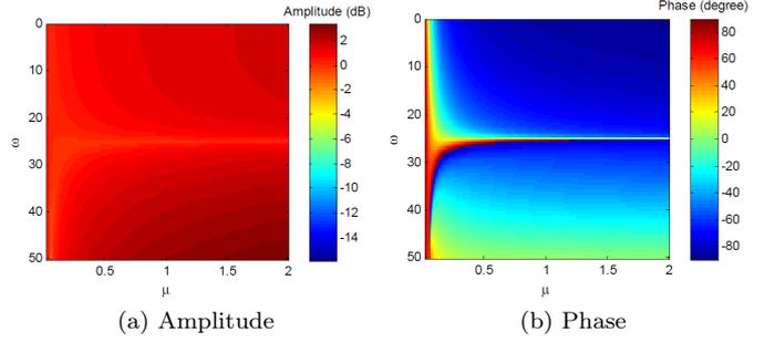
Fig. 5. Frequency characteristics of the additional controller dynamics for  $\omega \in [0, 30]$  for  $\mu \in [0, 2]$
