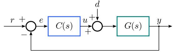
Fig. 1. Block diagram of a negative unity feedback control system with additive input disturbance
