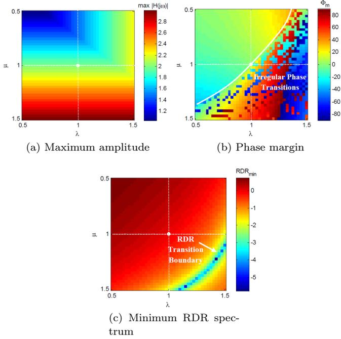
Fig. 4. Frequency characteristics of the controllers for  $\omega \in [0, 30]$  with an increment of  $0.01\text{rad/s}$
