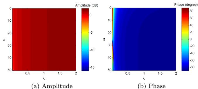
Fig. 6. Frequency characteristics of the additional controller dynamics for  $\omega \in [0, 30]$  for  $\lambda \in [0, 2]$
