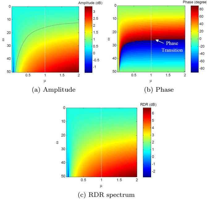
Fig. 2. Frequency characteristics of the controllers for  $\omega \in [0, 50]$  with an increment of 0.1rad/s versus  $\mu \in [0, 2]$  with 0.002 increments
