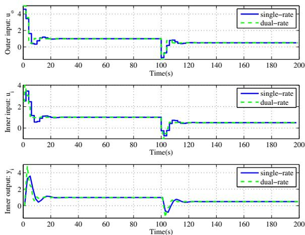
Fig. 9. Outer loop input and inner loop input/output for fast model
