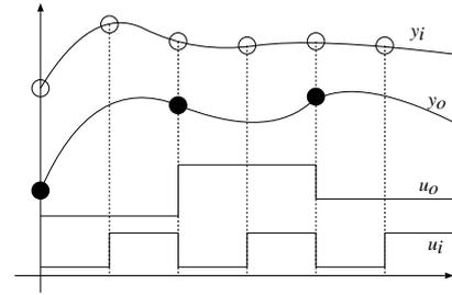
Fig. 3. Dual-rate input and output intervals
