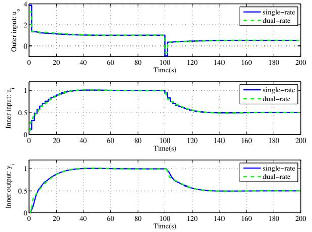
Fig. 7. Outer loop input and inner loop input/output for slow model
