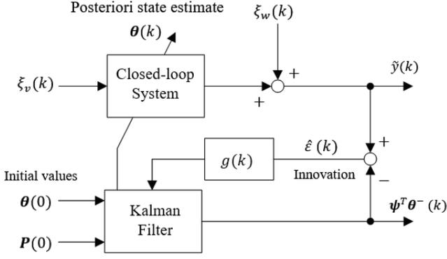
Fig. 1. Block diagram of proposed parameter estimator based on Kalman filter.
