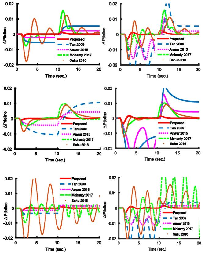
Fig. 7 (a-f). Tie line power deviation for (a,d) nominal, (b,e) lower bound, and (c,f) upper bound system parameters, for (a-c) without and (d-f) with, GRC and GDB respectively.
