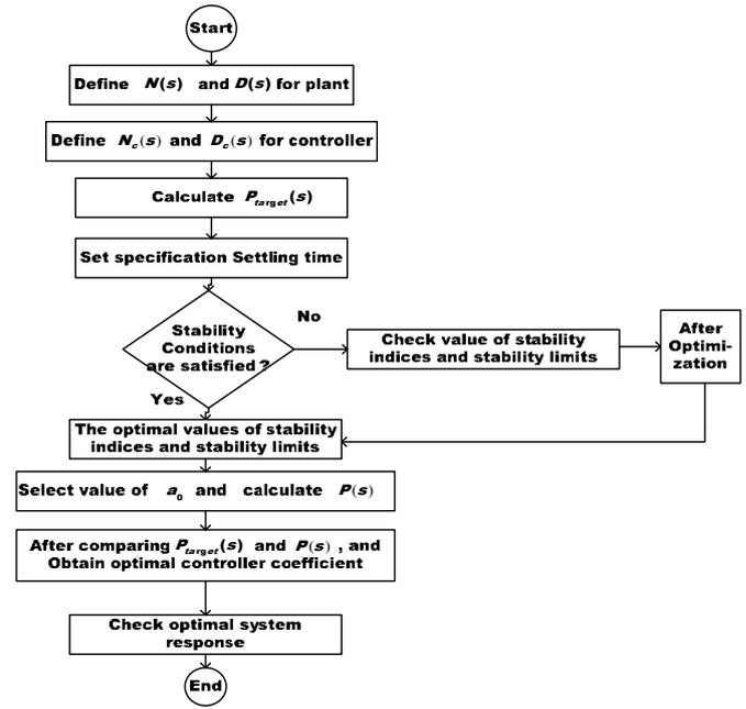
Fig. 2. Simplified flowchart for Coefficient Diagram Algorithm
