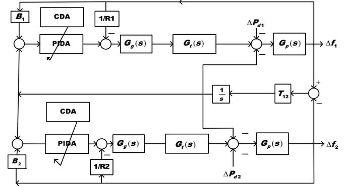
Fig. 4. The two area power system configuration with CDA-PIDA.
