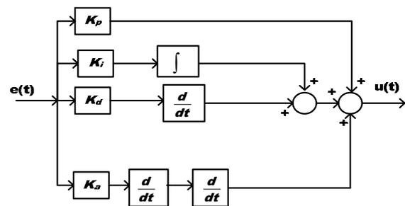
Fig. 3. The structure of PIDA Controller
