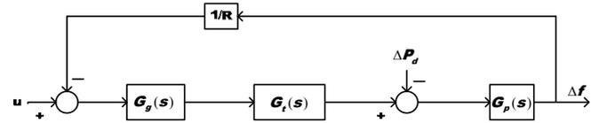
Fig. 1. Block diagram of single area power system.
