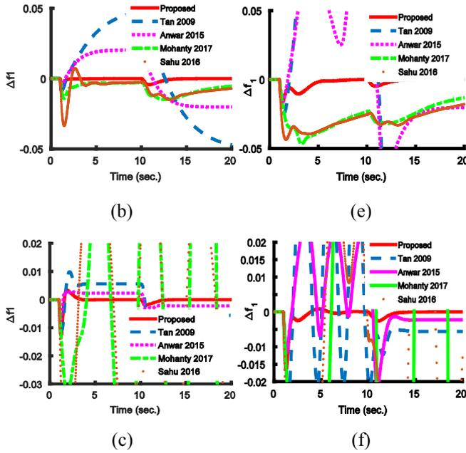
Fig. 5 (a-f). Frequency deviation in area 1 for (a,d) nominal, (b,e) lower bound, and (c,f) upper bound system parameters, for (a-c) without and (d-f) with, GRC and GDB respectively.
