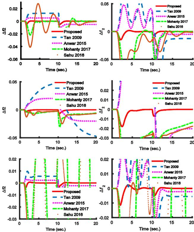
Fig. 6 (a-f). Frequency deviation in area 2 for (a,d) nominal, (b,e) lower bound, and (c,f) upper bound system parameters, for (a-c) without and (d-f) with, GRC and GDB respectively.
