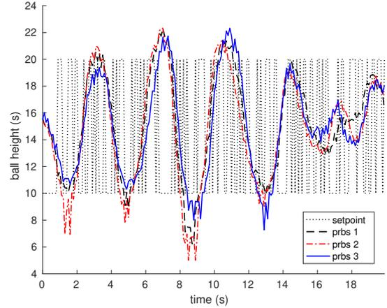
Fig. 2. An excerpt of the response to a PRBS input of amplitude 10cm applied to the setpoint.
