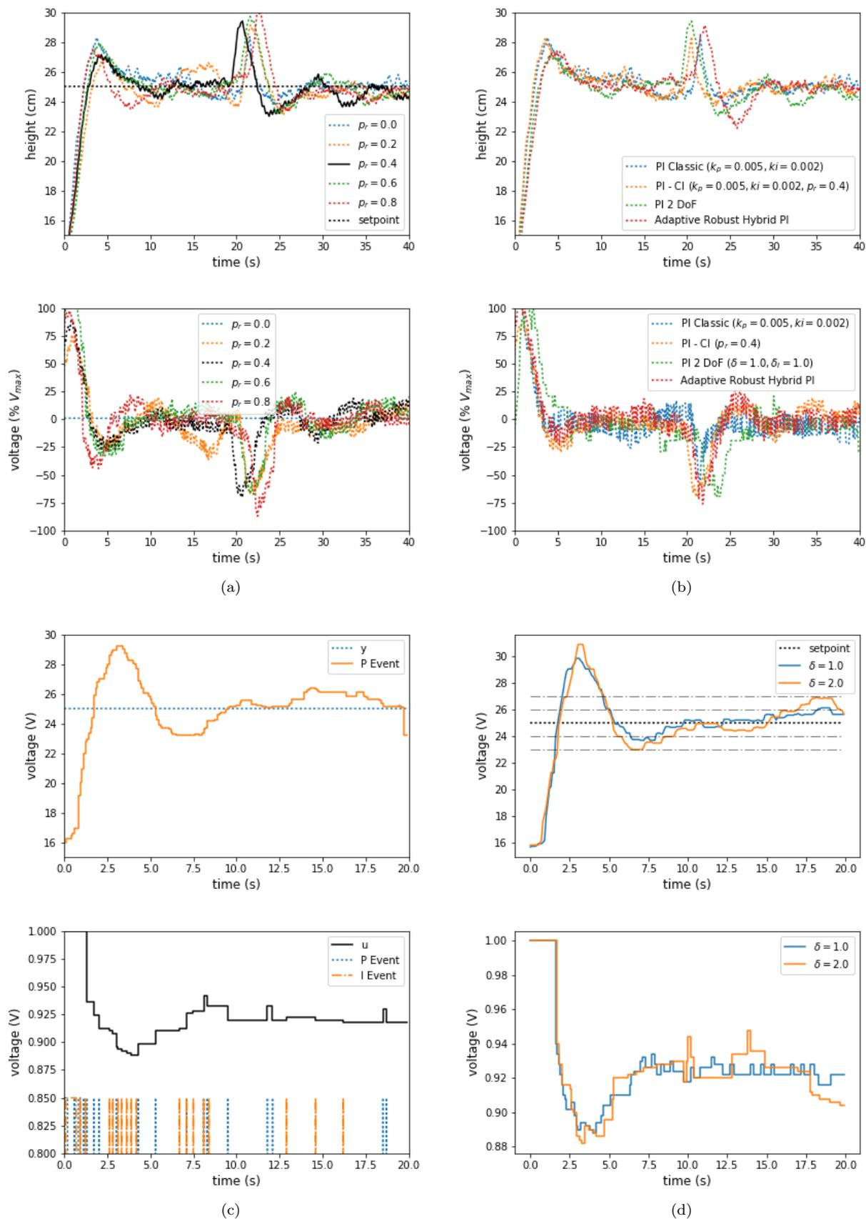
Fig. 4. (a) Step response of the PI-CI controller with  $k_p = 0.005$  and  $k_i = 0.002$ , varying the reset action  $p_r$  between 0 and 1, (b) step response of the four controllers with  $k_p = 0.005$  and  $k_i = 0.002$ , (c) Proportional and Integral Events, and (d) effect of  $\delta_P$  and  $\delta_I$  in the response.
