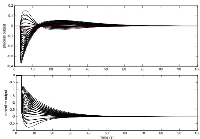
Fig. 11. Time domain simulations for nominal control design (Guzmán and Hägglund, 2011). A unitary step disturbance was included at time  $t = 3$  seconds
