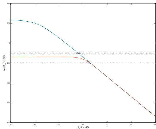
Fig. 2. Crossections for the regulation problem for  $FF = 0$  (red) and for  $FF \neq 0$  (blue) for  $\omega = 1$  rad/s and  $phase(L_0(j\omega)) = -100$  degrees. Two specifications are shown, for  $\delta_{dB} = -20$  (-) and  $\delta_{dB} = -10$  (-).
