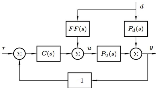
Fig. 1. Classical feedforward control scheme.
