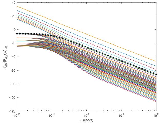
Fig. 4. Right side of Eq. (13) with  $FF = 0$  (\*) and with  $FF \neq 0$  (-) for nominal models  $P_u^0$  given by  $k_u = 1$  and  $\tau_u = 10$  and  $P_d^0$  given by  $k_d = 3$  and  $\tau_d = 11$ .
