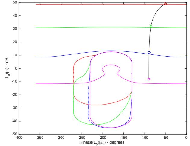
Fig. 7. Nominal open-loop shaping and stability and disturbance on output rejection bounds taking the FF element into account.
