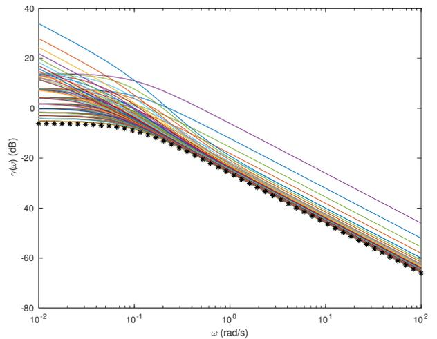
Fig. 5. Right side of Eq. (13) with  $FF = 0$  (\*) and with  $FF \neq 0$  (-) for nominal models  $P_u^0$  given by  $k_u = 10$  and  $\tau_u = 1$  and  $P_d^0$  given by  $k_d = 3$  and  $\tau_d = 11$ .
