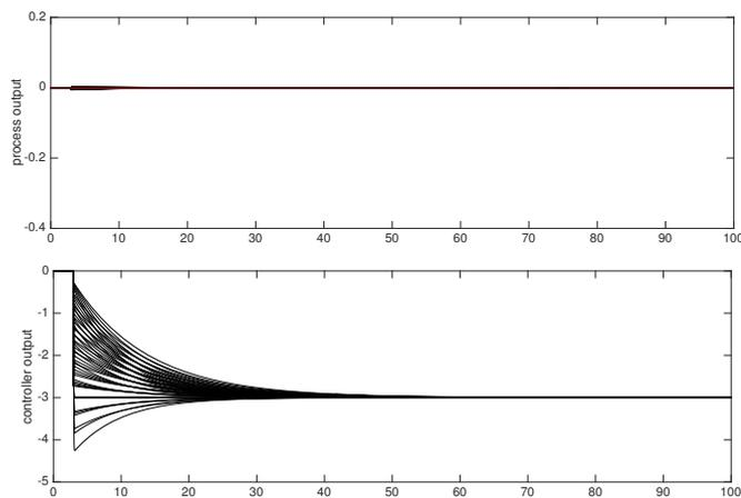
Fig. 10. Time domain simulations for the proposed robust control design. A unitary step disturbance was included at time  $t = 3$  seconds
