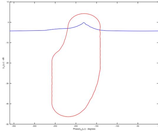
Fig. 3. Boundary comparisons for the regulation problem for  $FF = 0$  (red) and for  $FF \neq 0$  (blue) for  $\omega = 1$  rad/s and  $phase(L_0(j\omega)) = -100$  degrees and for the specification  $\delta_{dB} = -10$ .
