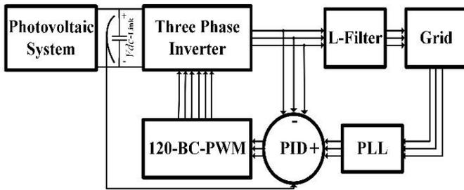
Fig.1. Block diagram of a three phase photovoltaic system.
