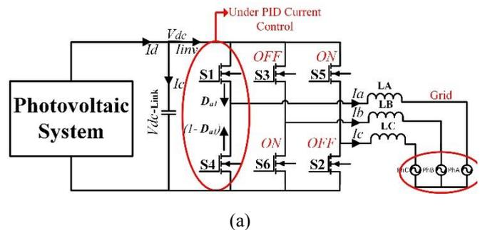
Fig. 5. Configuration of 120° BC-PWM under PID current control method.
