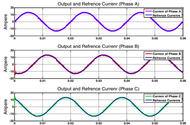
Fig. 9. Three phase measuring current and reference current
