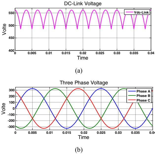
Fig. 3. DC-Link voltage: (a) dc link voltage  $V_{dc}$ ; (b) three phase grid voltage.
