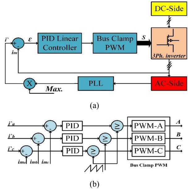
Fig. 4. Basic PID bus clamp current control theory: (a) Full control system; (b) PID and BC-PWM system.
