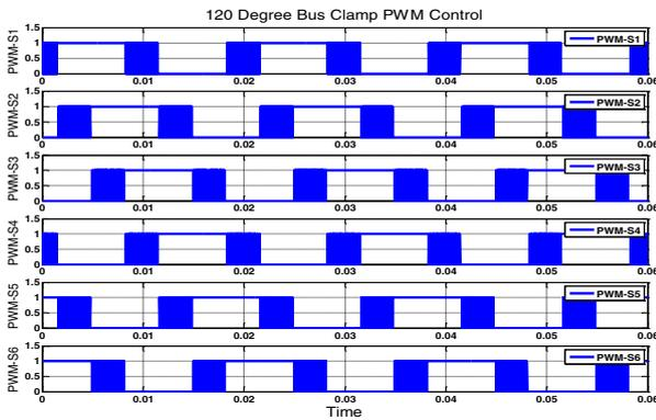
Fig. 6. Six PWM under BC-PWM and PID current control.
