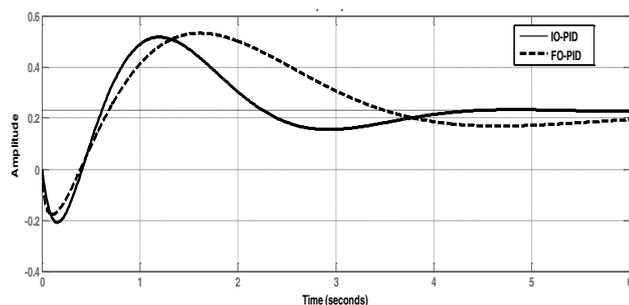
Fig. 7 Output response  $y(t)$  of the system after trade-off made for  $f_3(x)$
