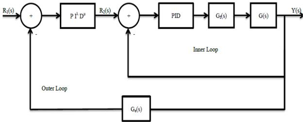
Fig. 1. Block diagram of PID-  $PI^\lambda D^\mu$  cascaded system
