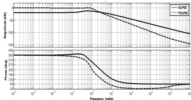
Fig. 8 Frequency plot after trade-off for best solution of  $f_1(x)$
