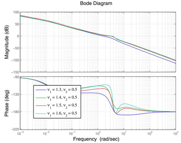
Fig. 3. Bode diagrams of the open-loop transfer function  $G_{OL2}(j\omega)$  in the outer loop, including the FOPI controller  $C_2$  and the inner feedback system  $G_{FOS}(j\omega)$  resulting from the FOPI controller  $C_1$
