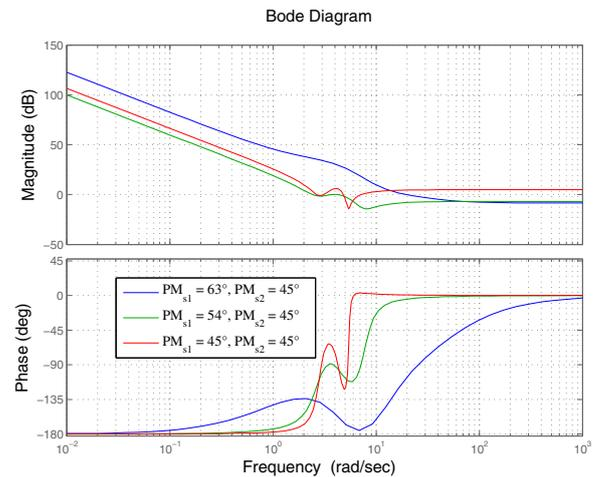
Fig. 4. Bode diagrams of  $G_{OL2}(j\omega)$ , including the PID controller  $C_2$  and the inner feedback system  $G_{IOS}(j\omega)$  resulting from the PID controller  $C_1$
