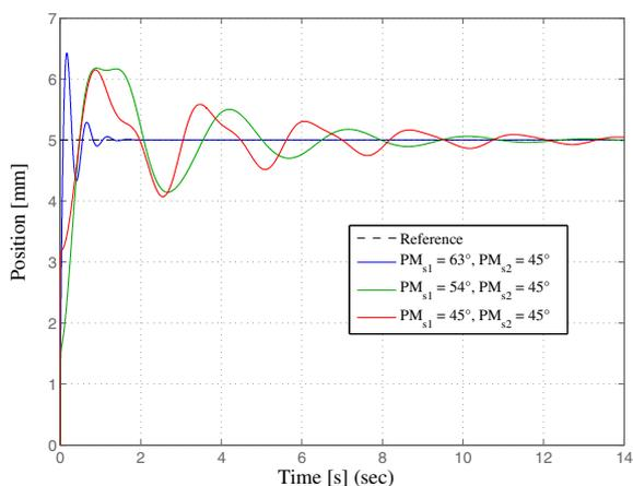
Fig. 7. Position output under PID control
