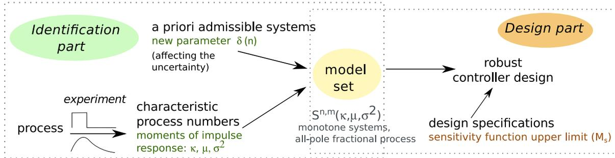
Fig. 1. Principal idea of the controller design based on the model set approach.
