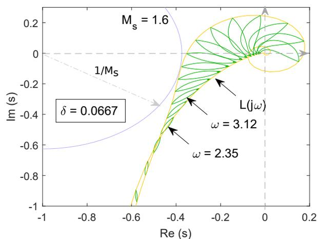
Fig. 7. Example: Nyquist plot plane for  $\delta = 0.0667$  ( $n = 30$ ) for normalized controller parameters
