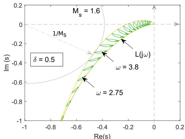
Fig. 6. Example: Nyquist plot plane for  $\delta = 0.5$  ( $n = 4$ ) for normalized controller parameters
