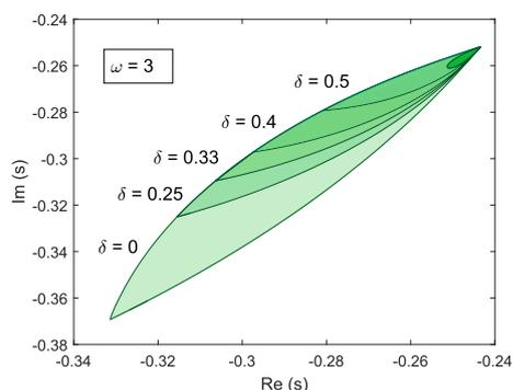
Fig. 8. Example: value set size shaped by new tuning parameter  $\delta$ , for frequency  $\omega = 3$  and  $\bar{\sigma}^2 = 0.34$
