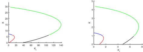
Fig. 2. Examples of robust regions curves in  $K_I - K$  plane, left for  $\delta = 0.25, \sigma^2 = 0.8$ , right for  $\delta = 0.1, \sigma^2 = 0.3$ . The red lines contain the optimal solution minimizing (6).
