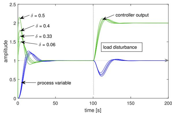
Fig. 9. Example: closed loop step responses and load disturbance responses dependent on  $\delta$
