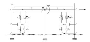
Fig. 1. Half-car semi-active suspension schematic
