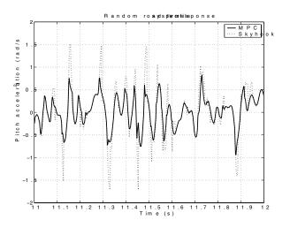
Fig. 4. Random profile. Up: Sprung mass barycenter heave acceleration. Down: Sprung mass barycenter pitch acceleration.
