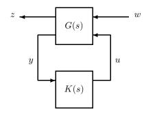
Fig. 1. Standard Feedback System
