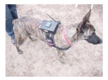
Figure 1. Remotely Commanded K-9 with Radio and GPS/INS Receiver
