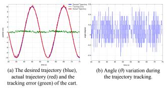
Fig. 5. Experimental results for point  $T_2$  ( $\tau_1 = 54 \text{ ms}, \tau_2 = 48 \text{ ms}$ ).
