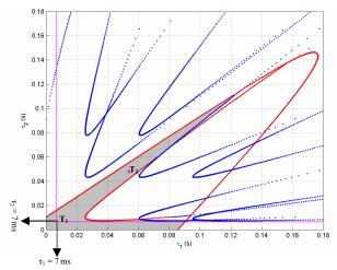
Fig. 3. The complete stability map of the multiple time-delayed cart-pendulum system in the domain of the delays.
