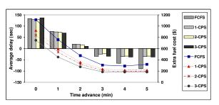
Fig. 8. Average delay (columns) and extra fuel cost (lines) vs. allowed time advance for the time interval 8-9AM.
