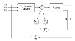
Fig. 2: Feedworward nonlinear control
