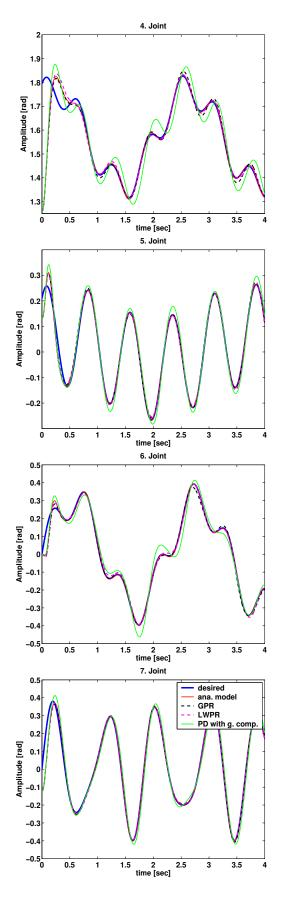
Fig. 5: Tracking performance for joint 4, 5, 6 and 7 with feedforward control using test trajectory.
