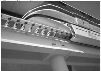
Figure 1 ODU Maglev Vehicle on Guideway
