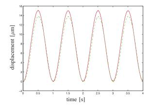
Fig. 13. Open-looped tracking of a 1 Hz sinusoidal reference (dotted line) with and without the compensation algorithm (continuous and dashed line).
