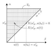
Fig. 7. Inverse Preisach model principle when  $\dot{u}(t) < 0$ .
