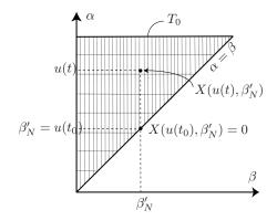
Fig. 6. Inverse Preisach model principle when  $\dot{u}(t) > 0$ .
