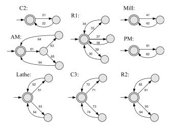
Fig. 6. Automaton models of plant components
