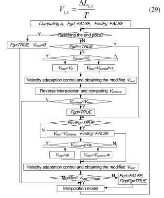
Fig.4 flowchart of pre-interpolation linear acc/dec of NURBS curve
