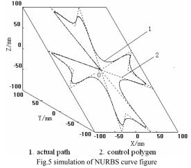
The NURBS simulation curve which is generated by the new second-order de Boor algorithm is shown in Figure 5. The NURBS curve is drawn in a three-axis x-y-z coordinate system. In this figure, 1 is the NURBS curve using the parameters in Table 1, while 2 is from the original control polygon whose vertexes are control points.
