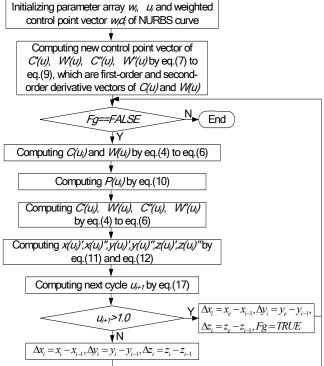
Fig.1 The flowchart of NURBS curve real-time de Boor interpolation algorithm
