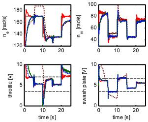
Figure 4: Closed loop response;  $u_m \approx u$  (solid red),  $\Lambda = 0$  (dotted dark red),  $\Lambda_{s3}$  (solid green),  $\Lambda_{d3}$  (dotted blue)
