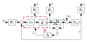
Figure 3: Anti-windup closed loop system
