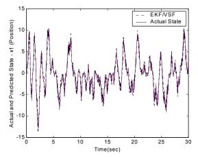
Figure 4a: Estimated and Actual States Associated with Modeling Error (Position)
