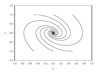
Fig.2. Phase portrait of PI controlled level process (underdamped).
