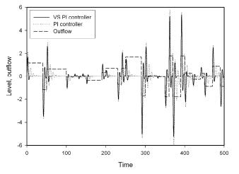
Fig.9. Level response to random step changes in outflow for IAE optimized PI control and IAE optimized VS PI control.
