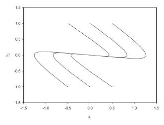
Fig.3. Phase portrait of PI controlled level process (overdamped).
