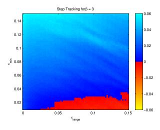
Fig. 4. Cost comparisons via subtraction for step tracking with  $\beta = 3$ . Positive values indicate SP-PB shows superior performance.
