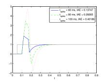
Fig. 7. Step responses for three delay spikes. Here, T=0.1 and  $\tau_{pb}=50$  ms.
