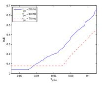
Fig. 8. Delay-spike cost as a function of the delay for three values of  $\tau_{pb}$ .
