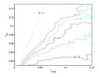
Fig. 5. Curves of equal cost for the unbuffered PID controller and the SP-PB. For all values of  $\beta$ , the area below and to the right of the curves is where the unbuffered PID controller has superior performance.
