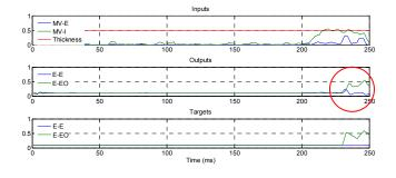
Fig. 7 Inputs, outputs and targets of EN-E generated during a DB-EO degraded cutting regime: range [0.1-0.9].
