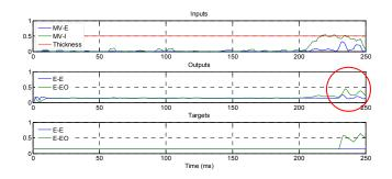
Fig. 6 Inputs, outputs and targets of EN-E generated during a DB-EO degraded cutting regime: range [0.15-0.85].
