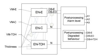
Fig. 2 Scheme of the recurrent neural network approach.
