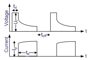
Fig. 1 Theoretical discharges of the WEDM process.
