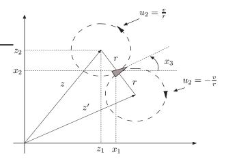
Fig. 1. Unicycle Circular Motion
