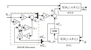
Fig. 4. Piecewise Continuous Reduced Order Luenberger Observer
