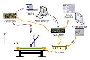
Fig. 1. Vision based inverted pendulum control system
