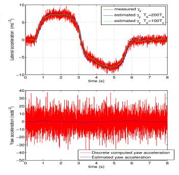
Fig. 1. Lateral acceleration filtering with 2 different window sizes (top). Comparison between a standard numerical differentiation of  $\dot{\psi}$  and the one obtained with the algebraic methods (bottom)
