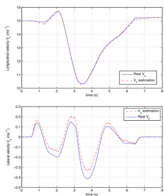
Fig. 5. Real and estimated longitudinal (top) and lateral (bottom) velocities with a friction coefficient  $\mu=0.7$
