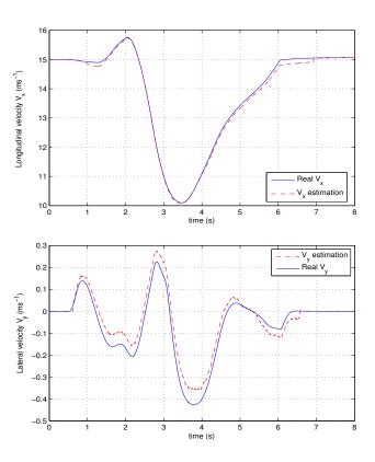
Fig. 6. Real and estimated longitudinal (top) and lateral (bottom) velocities with a friction coefficient  $\mu=0.9$
