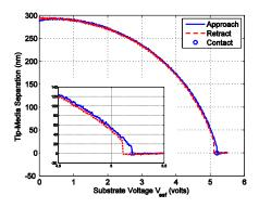
Fig. 6. A force/distance curve obtained by applying electrostatic force on the cantilever.
