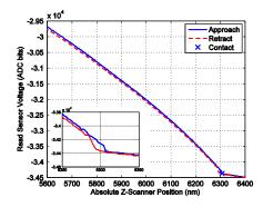
Fig. 5. A force/distance curve obtained by moving the z-scanner. The readback signal is a nonlinear function of the tip-medium separation, which can be approximated by a second-order polynomial.
