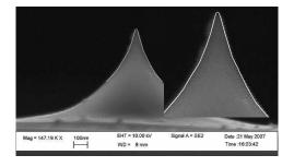
Fig. 9. Scanning electron microscopy image of a tip after tip wear experiment and the tip shape in white line before the experiment
