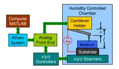
Fig. 2. Schematic of a single-lever data storage setup that serves as the development platform for a MEMS-based ultrahigh-density data-storage system.
