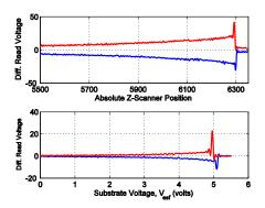
Fig. 7. During force/distance curve experiments using (top) z-scanner and (bottom) electrostatic force, peaks in the numerical derivative of the read back signal appear when the tip-medium contact and out of contact points occur.
