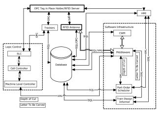
Fig. 4. Communication Flow of Testbed
