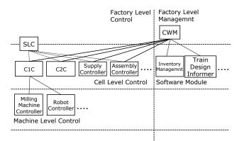
Fig. 2. ECA-Based Control Hierarchy of Testbed System
