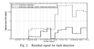
As it can be seen, the residual generated by the indirect design was not able to reflect the fault. But with performance improvement using interval division, the residual generator was able to detect the fault at the earliest possible time (10.4 sec).
