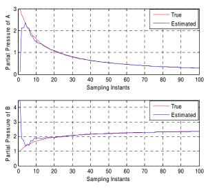
Figure 1: Evolution of true and estimated states of Partial pressures in Gas-phase reactor (CEnKF) (a) Partial Pressure of A (b) Partial Pressure of B
