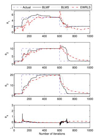
Fig. 6. Comparison between the proposed method (BLMF), the conventional BLMS, and EWRLS, L = 100.
