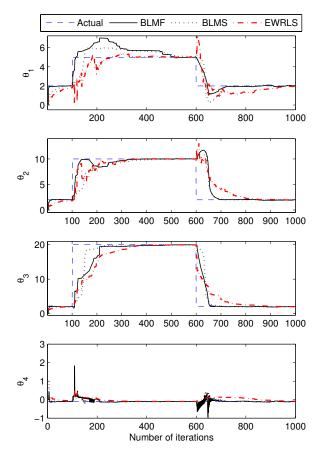
Fig. 5. Comparison between the proposed method (BLMF), the conventional BLMS, and EWRLS,  $L=50.\,$
