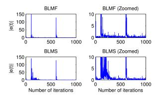
Fig. 2. Absolute Prediction error for BLMF and BLMS with optimal gain, L = 10. Right column shows the zoomed plots.
