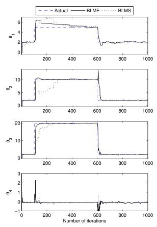
Fig. 1. Comparison between the proposed method (BLMF) and BLMS with optimal gain,  $L=10.\,$
