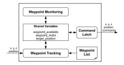
Fig. 9. Block diagram of the supervisory controller.
