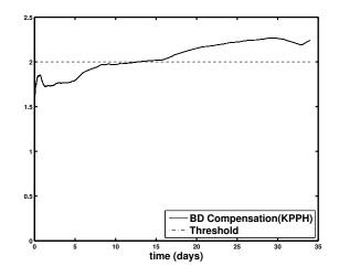
Fig. 2. Least Squares with Blowdown Compensation (Analysis result of real-time data during a period of a known tube leak).
