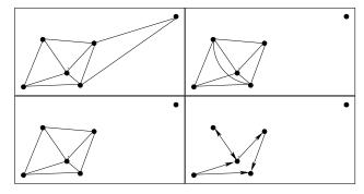
Fig. 2. From left to right, Delaunay graph, r-disk graph, r-limited Delaunay graph, and  $(r,\alpha)$ -limited wedge graph corresponding to the configuration in Fig. 1. The parameters are  $\alpha=\frac{\pi}{8}$  and r=0.5.
