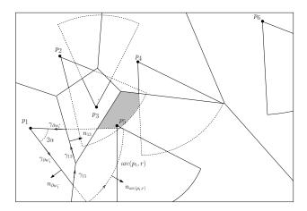
Fig. 1. Voronoi partition and wedge-shaped sensing regions corresponding to a random deployment of a robotic network. The parameters are  $\alpha =$ and r = 0.5. The notation for the various parameterizations of the Voronoi cell boundary and wedge sensing region are specified for robot 1.
