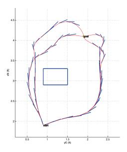
Fig. 9. Trajectories for the RH-CTG scheme in an obstacle field. All trajectories have the same starting state but each a different goal states are used (terminal heading  $\psi_{goal} = 0, \pi/2, \pi, -\pi/2$ ).
