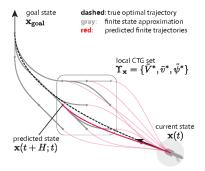
Fig. 3. Illustration of the RH+CTG optimization process.
