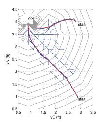
Fig. 5. Trajectory (in red) obtained from the RH+VF scheme with the VF shown in Figure 2 for a goal  $\mathbf{x}_{goal} = [4, 0]^T$ , and final states  $\psi_{goal} = 0$  and velocity  $u_{goal} = v_1 = 0.4$ m/sec. Also shown are the CTG points with associated states that were extracted along the way.
