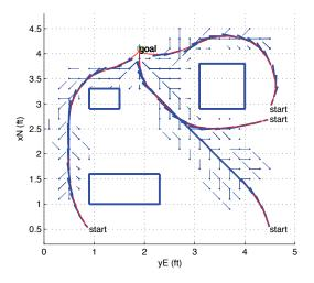
Fig. 8. Trajectories for the RH-CTG scheme in an obstacle field. The plot also shows the local VF points that were retrieved along the way.
