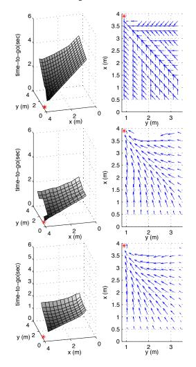
Fig. 7. Performance comparison of the control schemes: (top) only finite-state system; (middle) RH planner with cost-to-go; (bottom) nonlinear trajectory optimization with full horizon.
