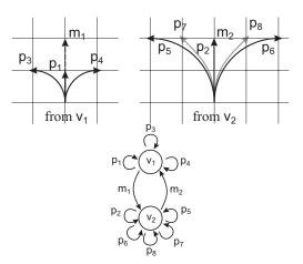
Fig. 1. (top) Illustration of an example motion primitive automaton (MPA). The motion primitives (MPs) are specified for quantized vehicle speeds. Transition between the speeds is enabled by acceleration and deceleration primitives. Each MPs trajectory segments start and end on a grid. (bottom) The transition graph of the MPA.
