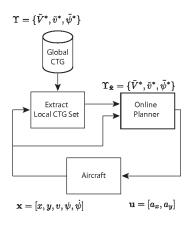
Fig. 4. Illustration of the receding horizon trajectory planning scheme with an approximate finite-state value function.
