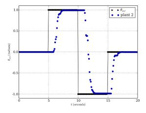
Fig. 8. Step response m=1 controller, (n-m)=(2-1)=1 perturbed plant,  $k_s=1$ , 76 meter spacing (high data dropout rate).
