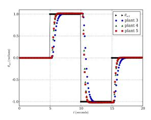
Fig. 6. Step response m=2 controllers, (n-m)=(5-2)=3 perturbed plants,  $k_s=\sqrt{\frac{5-2}{2}}$ , 70 meter spacing between radios.
