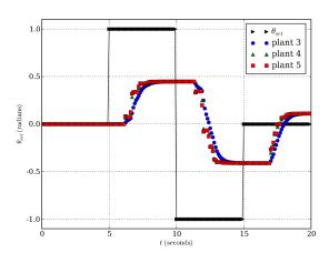
Fig. 7. Step response m=2 controllers, (n-m)=(5-2)=3 perturbed plants,  $k_s=\sqrt{\frac{5-2}{2}},\,74$  meter spacing (high data dropout rate).
