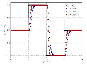
Fig. 5. Step response m=1 controller, (n-m)=(4-1)=3 perturbed plants,  $k_s=\sqrt{\frac{4-1}{1}},\ 70$  meter spacing between radios.
