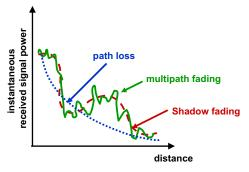
Fig. 4. A multi-scale representation of the received signal power
