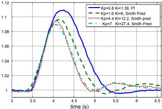
Fig. 4. Disturbance rejection with increasing gains: PI (bluesolid), moderate gain SP (green-dash), high gain SP (red-dot), very high gain SP (cyan-dash-dot).
