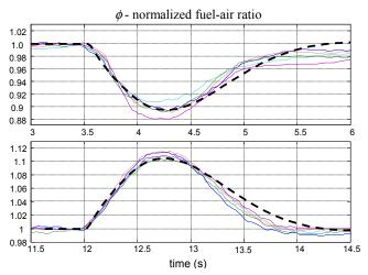
Fig. 1. Model (bold-dash curves) and repeated test responses to a 20% fuel-air ratio disturbance induced by changing injector slope.
