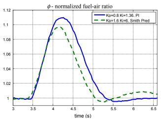
Fig. 3. Comparison of the Smith Predictor (green-dash) and the PI controllers (blue-solid) responses to a 20% FAR step disturbance.
