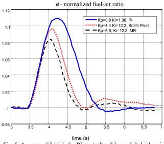
Fig. 5. Average of 5 trials for PI controller (blue-solid), high-gain Smith Predictor (red-dot) and MR controller (black-dash).
