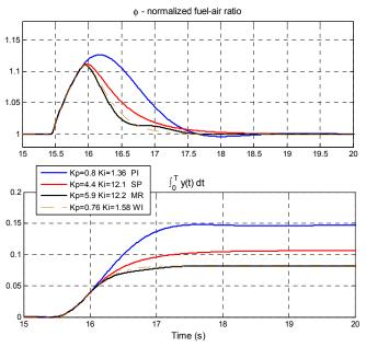
Fig. 6: Response to a 0.2 magnitude step disturbance (top plot) and its time integral (bottom plot) for PI, SP, and MR controllers plus the Watanabe-Ito controller (orange-dash dot).
