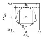
Fig. 4. Robustness ellipse in the plane of the uncertain disturbance parameters. Two constraints  $h_1$  (continuous line) and  $h_2$  (dashed line) are active for the robustly optimal process and control design.
