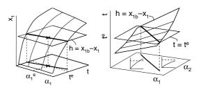
Fig. 2. Left: trajectories for different values of disturbance parameter  $\alpha_1$  and curve (thick line) connecting points where trajectories cross the boundary h = 0. Critical point at  $t^e, \alpha_1^e$  is marked by  $\times$ . Right: manifold of trajectories which fulfill constraint h = 0 at  $t^e$  after step disturbances of magnitude  $\alpha_1$  and  $\alpha_2$ . Sketches of trajectories show in which region h = 0 is crossed or not.
