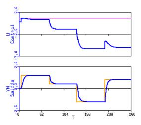
Fig. 9. Closed loop response of the asymmetric process to several step changes in the set point. Limits on *u*. Upper graph: control signal. Lower graph: set point and process output.
