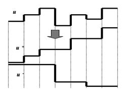
Fig. 3 Signal u(t) decomposed as  $u^+(t)$  and  $u^-(t)$
