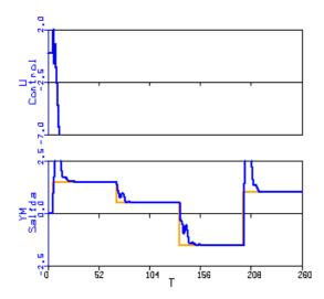
Fig. 13. Closed loop response of the asymmetric process to several step changes in the set point. Internal model  $G^{-}$ ,  $\beta = 0.1$ . Upper graph: control signal. Lower graph: set point and process output.
