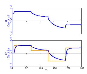
Fig. 12. Closed loop response of the asymmetric process to several step changes in the set point. Internal model  $G^+$  and  $\beta = 5$ . Upper graph: control signal. Lower graph: set point and process output.
