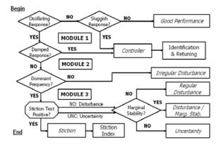
Fig. 2. Architecture of the CLPM system.
