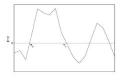
Fig. 4. Zero-crossing time for a half-cycle.
